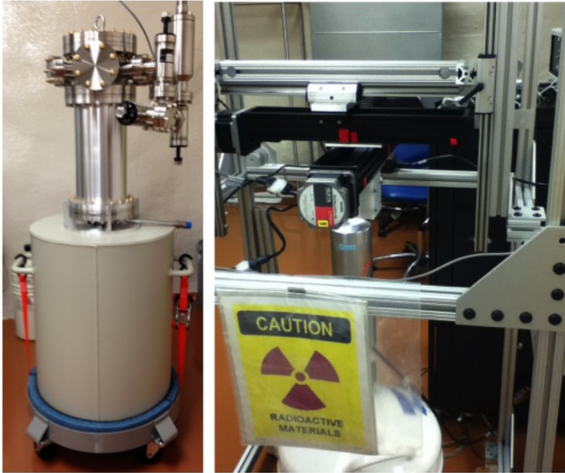
Fig. 4. Photos of the setups used in detector and string tests. Left photo: A string test cryostat attached to a dewar that provides liquid nitrogen cooling. Right photo: A HPGe detector in its PopTop™ cryostats is being calibrated using a collimated ^{133}\text{Ba} source. The source is mounted on an automated x-y scanner system that allows scans across the top of the detector. The scanner system can be reconfigured to allow scans in the z-direction.
