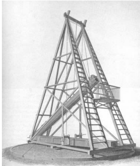
Figure 3: Ramage's 25-foot reflector erected in 1820 at Greenwich upon which the design of the mount for Mason's 12-inch telescope was based
