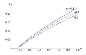
FIG. 5: Entanglement in the final state as a function of  $\eta_1$  for different values of  $\eta_2$ . Here  $1 - \eta_1$  and  $1 - \eta_2$  are the photon loss before and after the opto-mechanical system respectively. The values of the other parameters are  $N_D = |\alpha|^2 = 5000$ , r = 0.5, y = 0.1,  $N_{in} = 1$ ,  $\sigma = 0.01$ , x = 0.01,  $N_{th} = 10$ , and  $\eta_c = 0.8$ .
