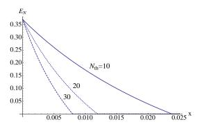
FIG. 4: Entanglement in the final state as a function of the mechanical noise parameter  $x = \gamma/G$ , for different values of the bath mean phonon number  $N_{th}$ . The values of the other parameters are  $N_D = |\alpha|^2 = 5000$ , r = 0.5, y = 0.1,  $N_{in} = 1$ ,  $\sigma = 0.01$ , and  $\eta_1 = \eta_2 = \eta_c = 0.8$ .
