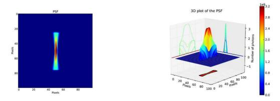
Figure 4. PSF of the petal made with Ge(111) without any misalignment errors in the positioning of the crystal tiles having no radial distortion.
