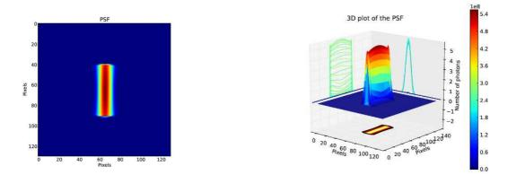
Figure 2. PSF of the petal made with GaAs(220) without any misalignment errors in the positioning of the crystal tiles having no radial distortion.
