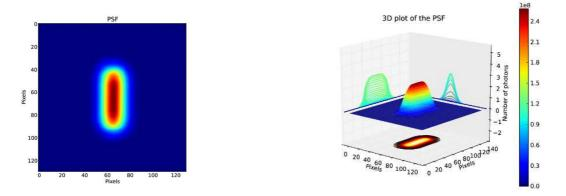
Figure 3. PSF of the petal made with GaAs(220) with a maximum misalignment of 30 arcsec in the positioning of the crystal tiles having a maximum radial distortion of 6 meters.
