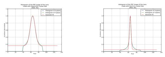
Figure 13. Histogram of the image PSF of the lens made by GaAs(220) crystal tiles (*left*), and that by Ge(111) crystal tiles (*right*). This lens is made with perfect positioning of the crystal tile, having no radial distortions.
