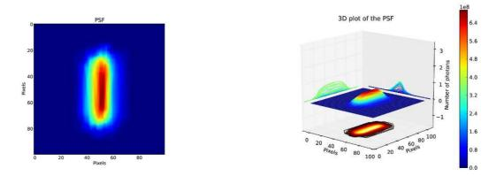
Figure 5. PSF of the petal made with Ge(111) with a maximum misalignment of 30 arcsec in the positioning of the crystal tiles having a maximum radial distortion of 6 meters.
