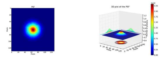
Figure 10. PSF of the lens made with Ge(111) with a maximum misalignment of 30 arcsec in the positioning of the crystal tiles having a maximum radial distortion of 6 meters.
