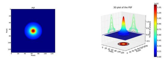
Figure 7. PSF of the lens made with GaAs(220) without any misalignment errors in the positioning of the crystal tiles having no radial distortion.
