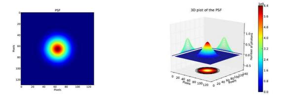
Figure 8. PSF of the lens made with GaAs(220) with a maximum misalignment of 30 arcsec in the positioning of the crystal tiles having a maximum radial distortion of 6 meters.
