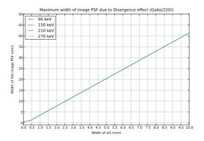
Figure 6. The effect of the divergence with the varying slit width (on the x - axis) on the FWHM of the image PSF.
