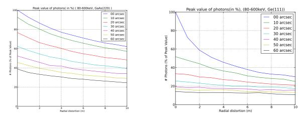
Figure 12. Peak intensity profile of the lens made with GaAs(220) (*left*) and Ge(111) (*right*) for different values of crystal misalignment and radial distortion. The values in the *legend* shows maximum misalignment (in arcsec) in the positioning of crystals.
