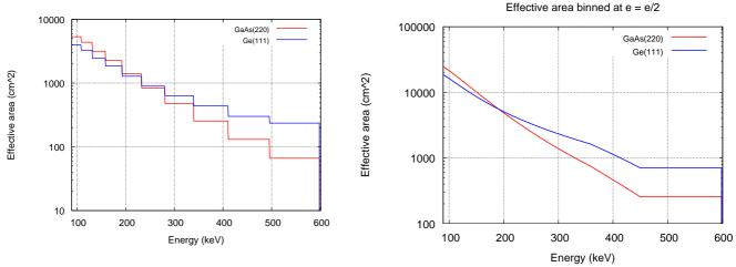
Figure 15. Effective area of the Lens made of GaAs(220) as well as Ge(111) crystal tiles calculated for 10 bins sampled equally in logarithmic scale (*left*) and for  $\Delta E = e/2$  right.
