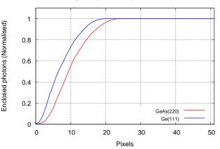
Radial profile (Normalised) of enclosed photons
