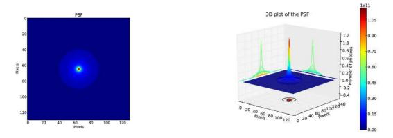
Figure 9. PSF of the lens made with Ge(111) without any misalignment errors in the positioning of the crystal tiles having no radial distortion.
