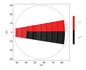
Figure 1. An illustration of the petal structure (that is being build in the LARIX facility) and the position of each crystal tile over it.
