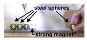
FIG. 5. The Gauss gun.
