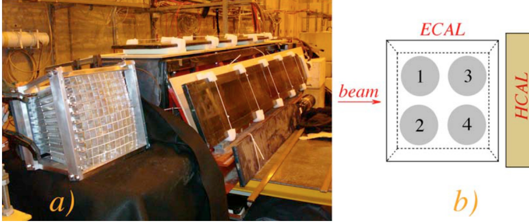
Figure 5: The 100-crystal BGO array placed in front of the DREAM module and exposed to electron and pion beams incident from the lower left in this photo.
