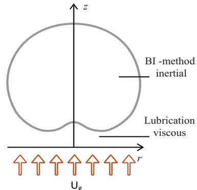
FIG. 2. Numerical implementation of the drop levitated by an airflow with uniform upward flow velocity  $U_g$ . The numerics consist of a coupling between the Boundary Integral method for the inviscid drop, and the lubrication approximation for the airflow beneath the drop. The flow inside the drop is assumed to be a potential flow; the flow at the bottom of the drop is a viscous flow, in which inertial effects are neglected.
