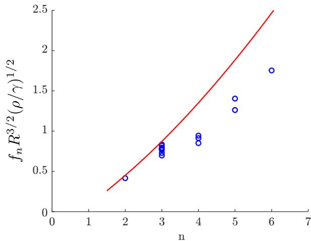
FIG. 6. The frequency measured for faceted drops as shown in the images of Fig. 5. Each data point  $\circ$ , corresponds to one water drop measurement. The red solid line is the prediction from the corresponding eigen mode for a puddle, given by eq. (2).
