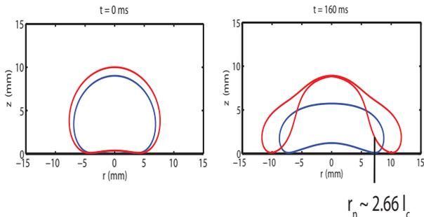
FIG. 11. Chimney instability. Shown is the evolution of two drops, with *almost* equal volumes. The largest drop apparently has a radius just above the chimney threshold, which appears to be about  $2.7\ell_c$ , or 7.3 mm, while the smallest has a radius just below. The large drop does not remain stable, due to the gas pocket breaking through; the small drop keeps its steady shape.  $Bo=2.25$  and  $2.5$ ,  $Ca=2.5 \cdot 10^{-5}$ ,  $\Lambda=11 \cdot 10^3$ .
