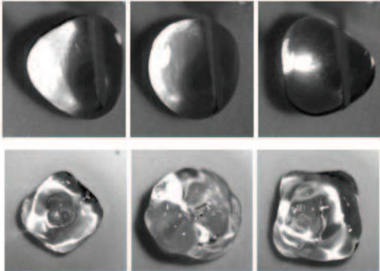
FIG. 1. Star drops levitated by a steady (i.e. non-pulsating) airflow. Top: mode  $n=3$ ; bottom: mode  $n=4$ . Figure from Ref. [12].
