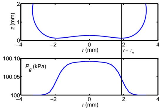
FIG. 10. Pressure profile ( $P_g$ ) at the bottom of a steady levitated drop. The largest pressure gradient is typically at the neck,  $r = r_n$ , such that the profile resembles a plateau.  $Bo=1$ ,  $Ca=2.5 \cdot 10^{-4}$ ,  $\Lambda=11 \cdot 10^3$
