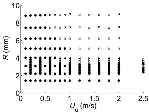
FIG. 15. Top view radius  $R$  versus airflow velocity  $U_g$  stability diagram for  $\Lambda=11 \cdot 10^3$ . Black dots point out stable configurations: the drop has no tendency to oscillate; white squares indicate oscillating drops.
