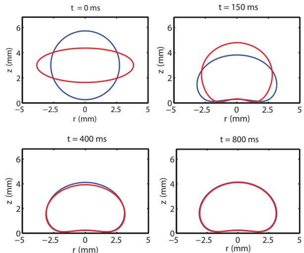
FIG. 9. Two different initial drop shapes (one spherical, one elliptical) of equal volume, converging to the same steady end shape.  $\text{Bo}=1$ ,  $\text{Ca}=2.5 \cdot 10^{-4}$ ,  $\Lambda=11 \cdot 10^3$ . See Fig. 10 for the corresponding pressure profile.
