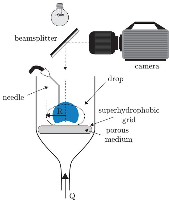
FIG. 3. Sketch of the experimental setup. Illumination and camera view are obtained using a beamsplitter. A flow rate  $Q$  is prescribed through a porous medium. Since the levitated drop is very mobile, it is held in position by a needle, which also supplies the liquid.
