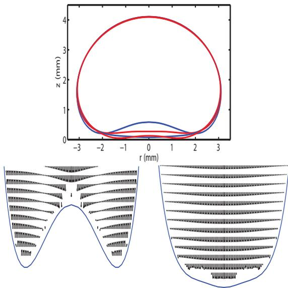
FIG. 13. Drop contours during the final stages of the simulation in an unstable scenario (see Fig. 12). Blue contours are the two extremes, red lines are intermediate. The bottom two plots show the velocity profile inside the drop for the extremes. Note that the liquid velocities, and therefore the oscillations as well, are mainly in the vertical direction.  $Bo=1$ ,  $Ca=2.5 \cdot 10^{-4}$ ,  $\Lambda=8.2 \cdot 10^3$ .
