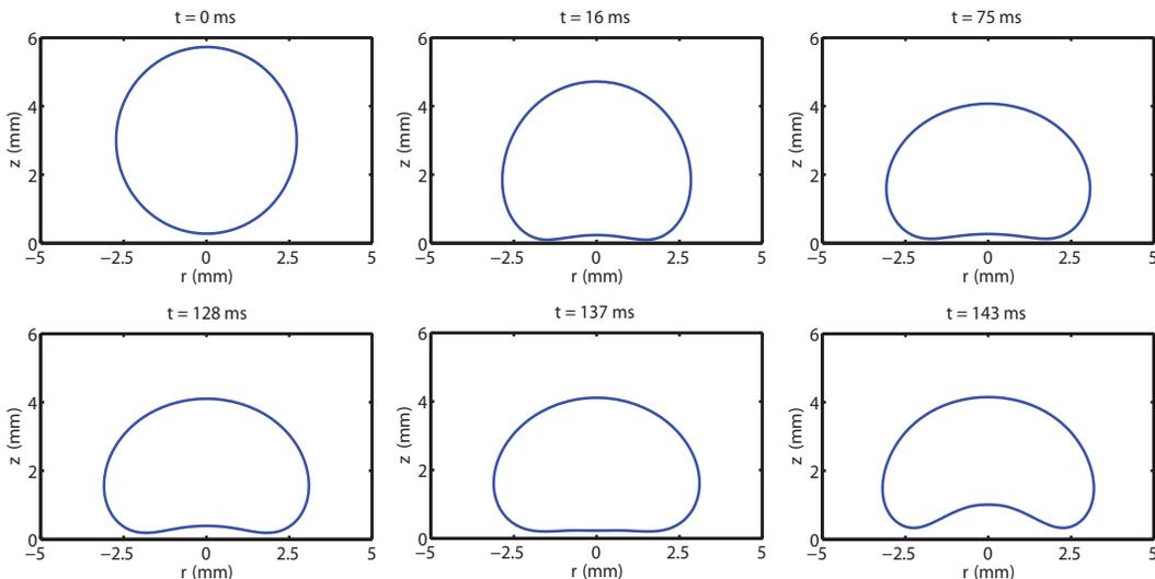
FIG. 12. Time sequence from the evolution of the oscillatory instability of a levitated drop. The simulation is initiated by a spherical drop, released from small height (0.27 mm) (top-left). The top panel row shows the process from the spherical drop shape to an intermediate steady shape. The bottom panel row shows the oscillatory behavior of the drop at a later point in time.  $Bo=1$ ,  $Ca=2.5 \cdot 10^{-4}$ ,  $\Lambda=8.2 \cdot 10^3$ .
