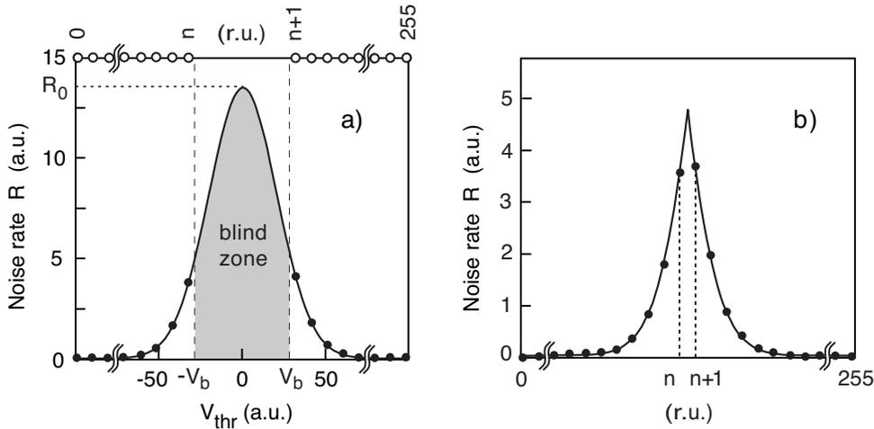
**Figure 3.** a): Noise counting rate of an ideal discriminator as a function of its threshold (continuous curve). With the CARIOCA discriminator the threshold values comprised in the shaded area cannot be set and the rate at zero threshold ( $R_0$ ) cannot be measured. In the upper scale the DAC registers which set the thresholds are schematically reported. b): Typical experimental curve representing the noise counting rate of a CARIOCA discriminator as a function of the DAC registers.
