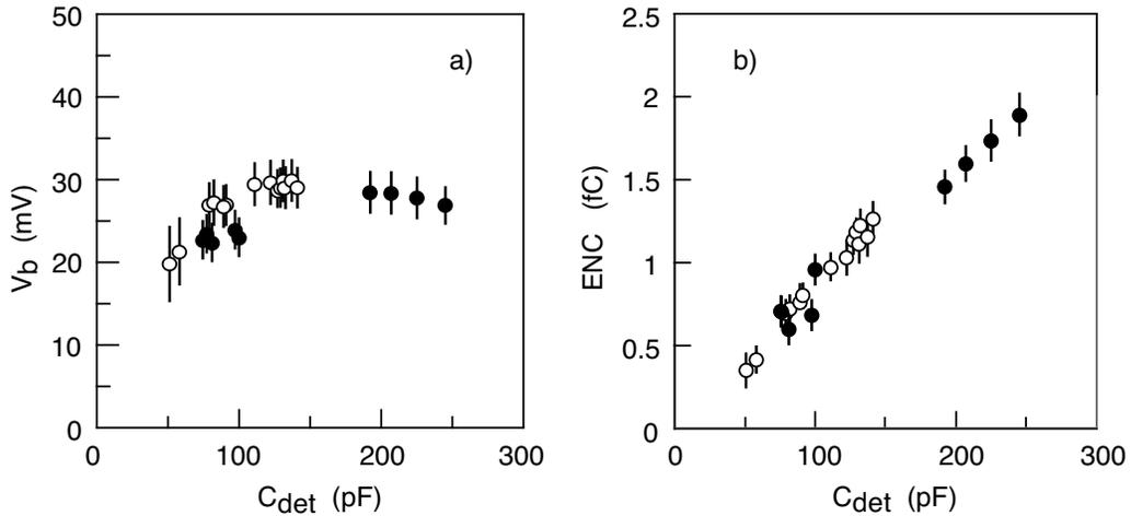
**Figure 10.** Dependence: a) of the bias voltage ( $V_b$ ) and b) of the ENC, on the detector capacitance. Open (full) points refer to cathode (anode) readout. The error bars represent the r.m.s. of the distributions.
