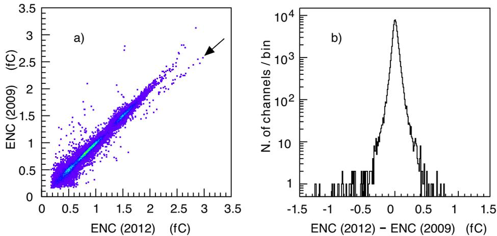
**Figure 11.** a): Scatter plot of the ENC values measured on all the muon detector in the years 2009 and 2012. The channels which are far from the plot bisector were checked and repaired or replaced. Most of the points in the series indicated by an arrow correspond to CARIOCAs mounted on the same boards which were replaced. b): Distribution of the difference between the ENC measured in 2012 and 2009.
