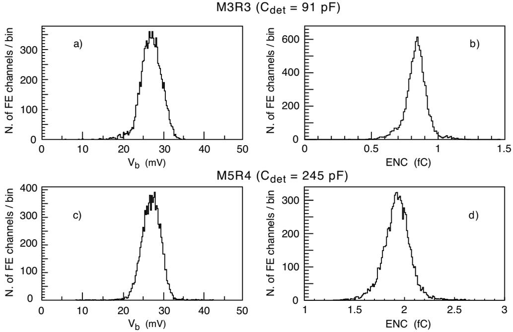
**Figure 9.** Distribution of: a) the bias voltage; b) the ENC measured for of all the readout channels of the region M3R3. c) and d): same as a) and b) for the readout channels belonging to region M5R4.
