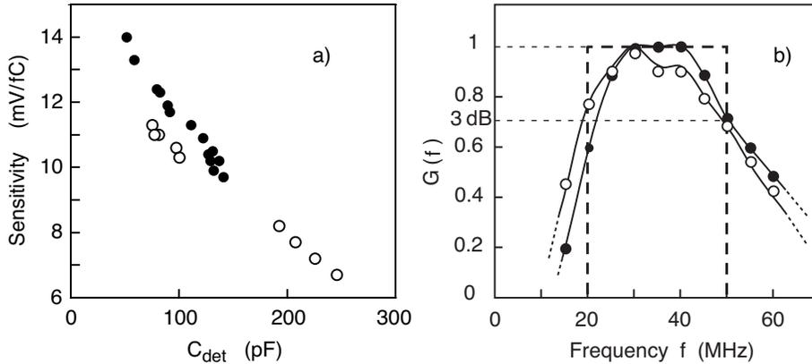
**Figure 1.** a): Measured sensitivity of the amplifier. b): Measured gain  $G$  of the amplifier for a sinusoidal signal as function of frequency  $f$ . The curves are normalized to their maximum value. The rectangular approximation to the frequency spectrum of the amplifier gain, as used in the MC simulation, is indicated with the 3dB limits at 20 and 50 MHz. The lines are to guide the eye. In both figures the open (full) points refer to negative (positive) input polarity.
