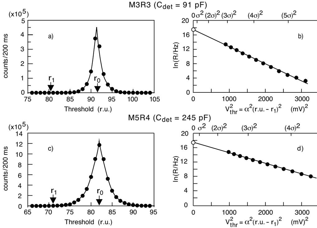
**Figure 8.** a): Experimental threshold scan of a readout channel of region M3R3. In b) the right-arm of this distribution is represented with logarithmic-quadratics scales. The open point at zero threshold is the counting rate predicted by Rice theory and by the MC. The straight line is the best fit to the points (see text). c) and d): same as a) and b) for a readout channel belonging to region M5R4. The larger detector capacitance ( $C_{det}$ ) results in a larger  $\sigma$ .
