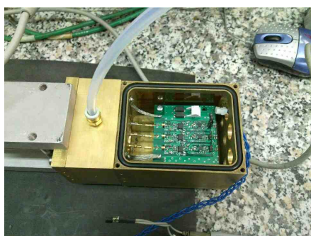
FIG. 31: Schematics of the front-end developed for the new MEG drift chamber
