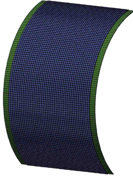
FIG. 70: Assembly of 93 PCB strips on the inner wall of the \gamma entrance window.
