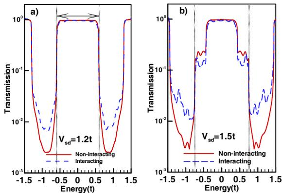
FIG. 6: The effect of electron-electron interaction in the mean-field level on transmission curves for two voltages a) NDR threshold voltage which is equal to  $1.2t$ , b) a voltage above the NDR threshold such as  $1.5t$ .
