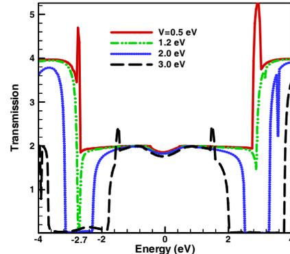
FIG. 9: Top: Zigzag graphene nanoribbon terminated by Hydrogen atoms. Bottom: First principle calculation of transmission through the above system as a function of energy for different values of external biases.
