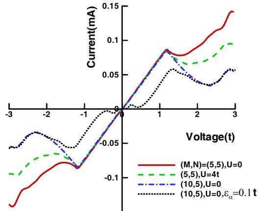
FIG. 2: Current-voltage characteristic curve of an odd zigzag graphene nanoribbon with  $N = 5$  (zigzag chains). I-V curves are compared for two ribbon lengths;  $M = 5$  and  $10$ . For the case of  $(M, N) = (5, 5)$  and for comparison purpose, I-V curve is also plotted in the presence of electron-electron interaction ( $U$ ) and asymmetric factor ( $\varepsilon_\alpha$ ).
