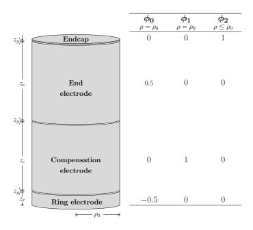
Figure 2: The trap geometry and boundary conditions used in the analytic solution.
