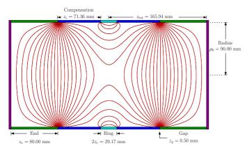
Figure 3: The optimized trap geometry with SIMION generated electric fields lines overlayed.
