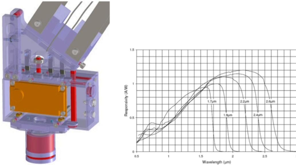
Figure 5: Left: Mechanical design of the receiver housing. The downward looking tube contains the collecting lens and a filter, the metal box houses the amplifier circuit. Right: Sensitivity curves for IR photodiodes. A cut-off of 2.2μm yields optimum sensitivity at the metrology wavelength of 1.9μm.
