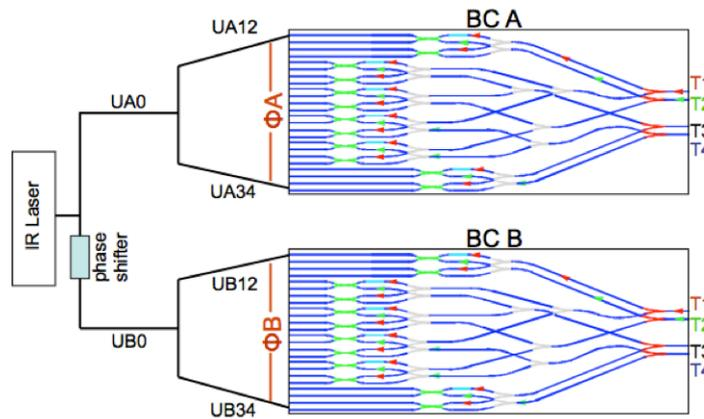
Figure 6: The non-common path, which enters the astrometric error budget, is  $(\Phi_A - \Phi_B)$  for the chosen injection scheme. Since the phase differences  $\Phi_A$  and  $\Phi_B$  occur in the two distinct spectrometers, each of them has to be kept stable to the nm-level.
