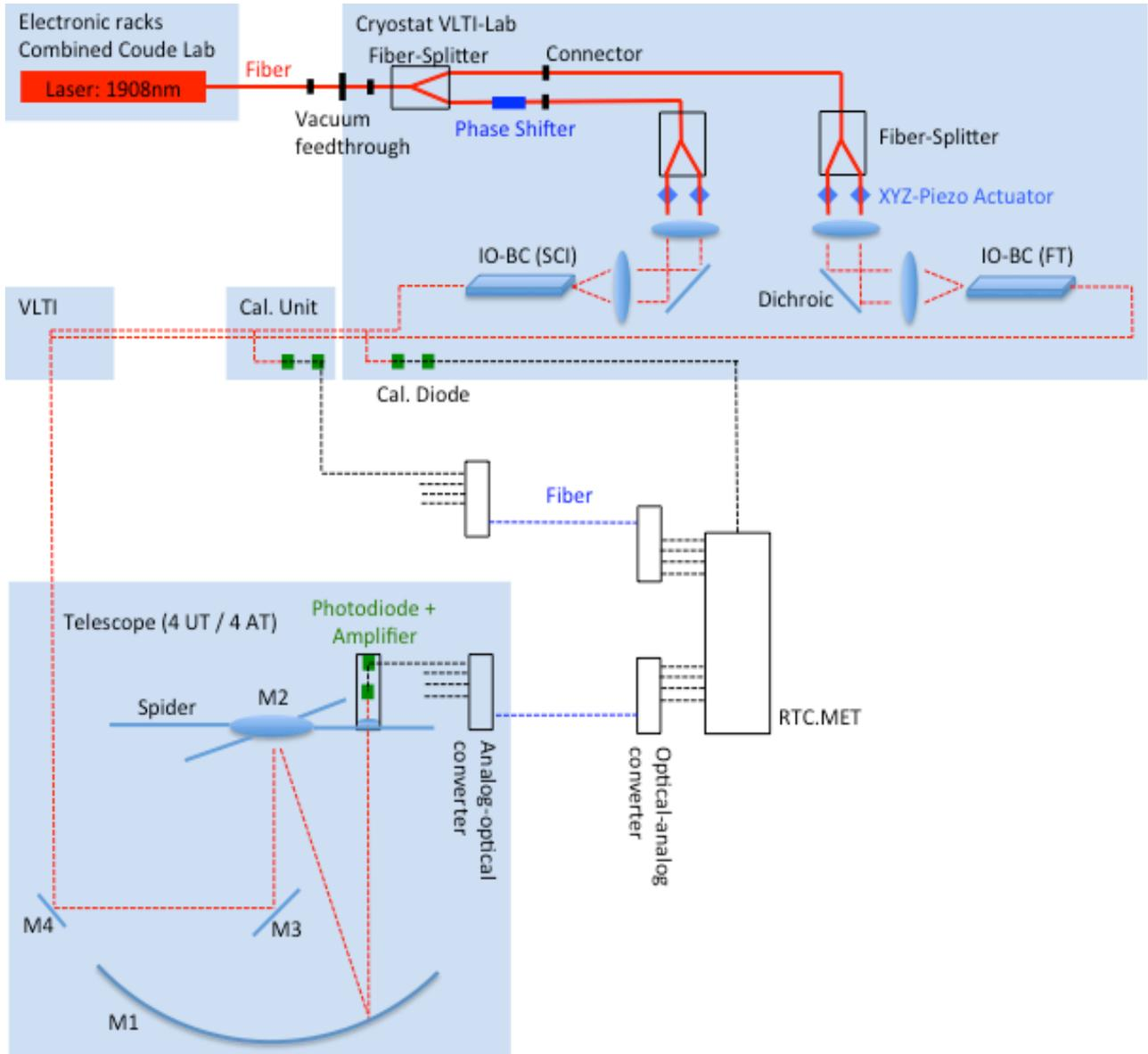
Figure 2: Schematic view of the implementation of the GRAVITY metrology
