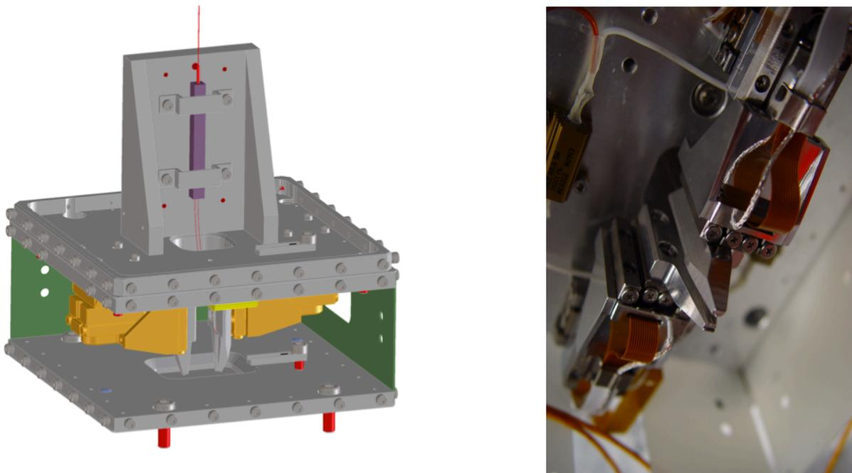
Figure 3: Left: Schematic view of the fiber injection unit with the fiber feeding the splitter from the top. Right: Photo of the fiber positioner prototype, showing the mounts into which the fibers are glued.
