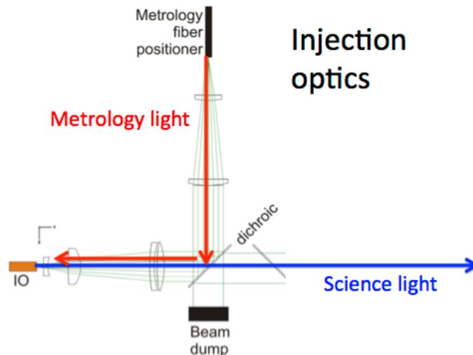
Figure 4: Optical layout of the injection unit.
