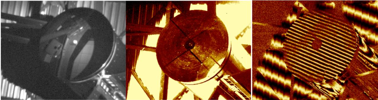
Figure 7: Testing the differential aberrations of the VLTI beam train. Left: view of the secondary mirror from below. Middle: The mirror is illuminated with metrology light from the VLTI lab, showing the spider arms and the central obscuration from a mask on M8. Right: Interferogram on the secondary mirror from which the aberrations can be determined.
