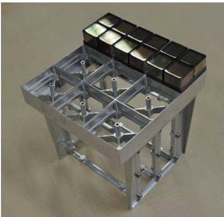
Figure 6. Prototype of the PDM Mechanical Structure with 12 MAPMTS
