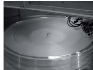
Figure 3. Fresnel Lens Machining
