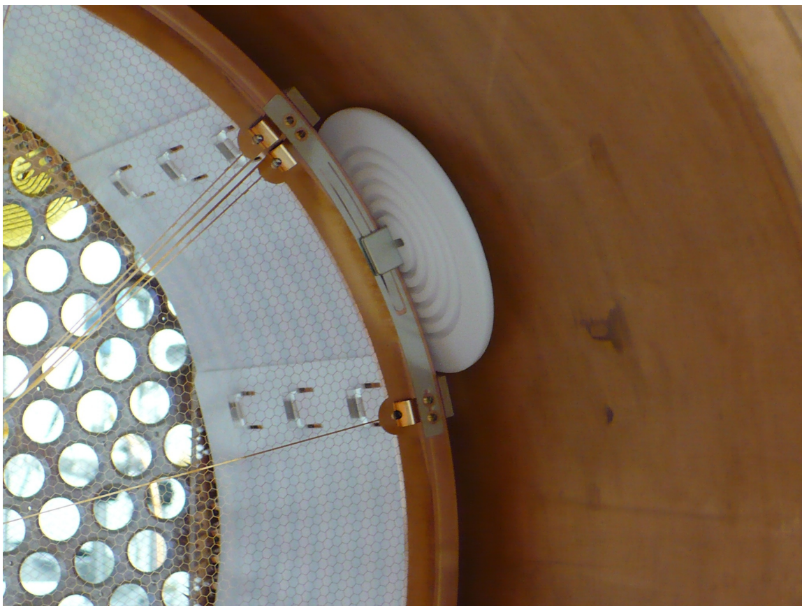
Figure 13. Platinum plated leaf spring connecting the HV feed to the cathode ring. The other field cage (with no cathode grid installed, is connected with a similar leaf spring).
