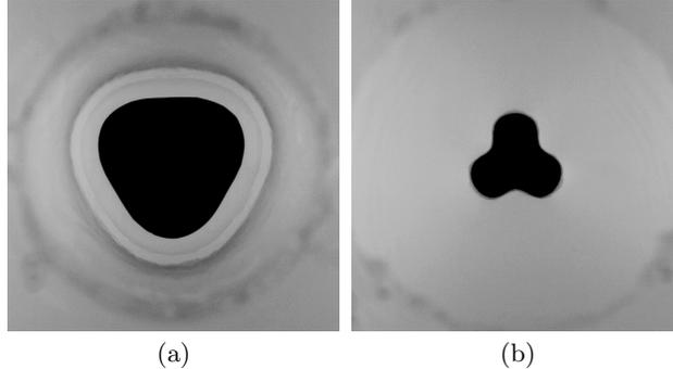
Figure 4: (movie online) Image of a  $m = 3$ ,  $R_{disc} = 20$  mm,  $a = 0.1R_{disc}$  cavity, approx. 10 ms after disc impact (a). Approximately 90 ms afterwards, it is clear that the shape has inverted with respect to the original (b).
