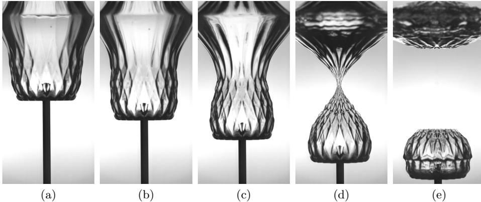
Figure 9: (movie online) Evolution of the collapse of an  $m = 20$ ,  $a_{20} = 4\%$  cavity as viewed from the side;  $R_{disc} = 20$  mm and  $V_0 = 1$  m/s.
