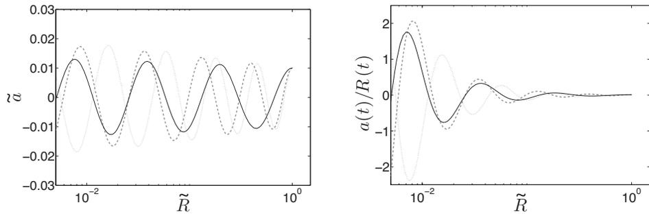
Figure 8: Theoretical behaviour of the amplitude, normalized by the disc radius, of a  $m = 20$ ,  $a_{20}(0) = 0.01R_{disc}$  collapse with different surface tension values (left). —  $\sigma = 0$ , — —  $\sigma_m = 47.1 \text{ mN/m}$  (milk),  $\cdots$   $\sigma_w = 72 \text{ mN/m}$  (water). The same plot is shown on the right, but with the amplitude  $a_{20}(t)$  divided by  $R(t)$ , to illustrate the growth of the relative disturbance.
