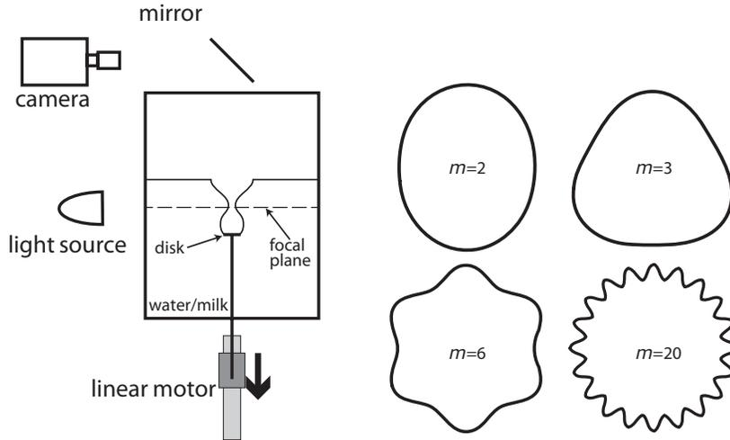
Figure 2: Experimental setup and examples of impacting discs. This camera-mirror configuration is used for top views; for side videos we simply move the camera down to the level where the light is. The shown discs have a disturbance amplitude of 10% of the mean radius ( $R_{disc}$ ).
