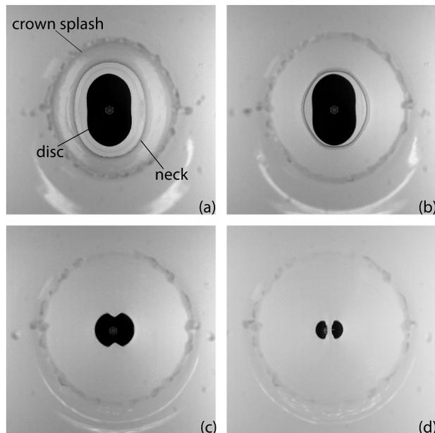
Figure 3: (movie online) Top view of a collapsing cavity ( $m = 2$ ,  $R_{disc} = 20$  mm  $a_2 = 0.25R_{disc}$ ) focused on the pinch-off plane. The cavity (neck) and the disc are initially in phase (a). Since the curvature is higher at the top and bottom of the neck, acceleration along the longer axis is larger. This changes the shape of the cavity as it collapses (b and c). Finally, the two points that were originally farthest apart come into contact first (d).
