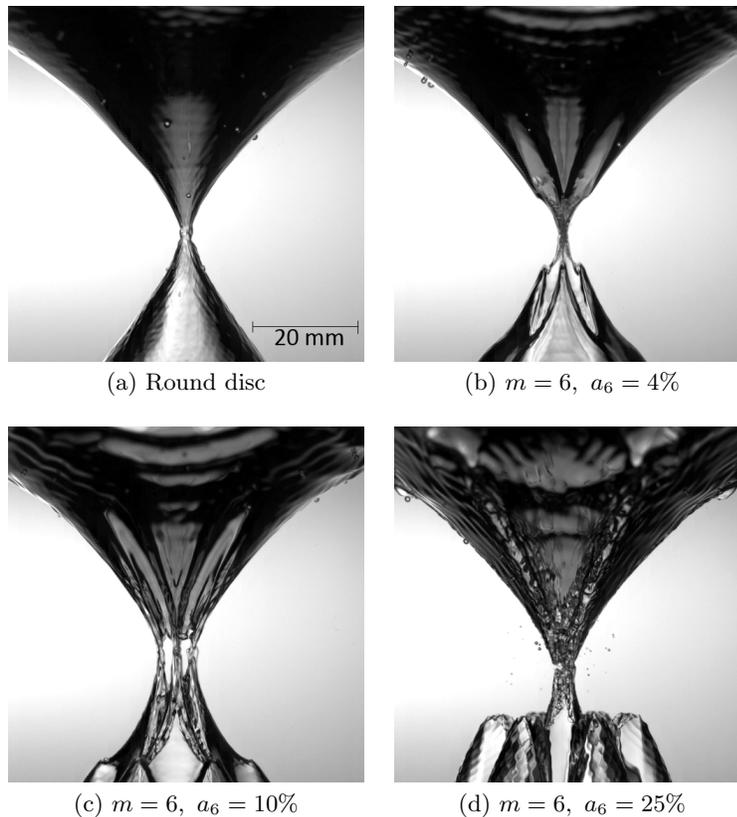
Figure 13: (movie online) Effects of axial symmetry breakup on pinch-off. Perturbed cavities no longer collapse at the same point and, as could be expected, the effects become more pronounced with larger amplitudes. Up-down asymmetry is noticeably accentuated, affecting more the void below the deep seal point.
