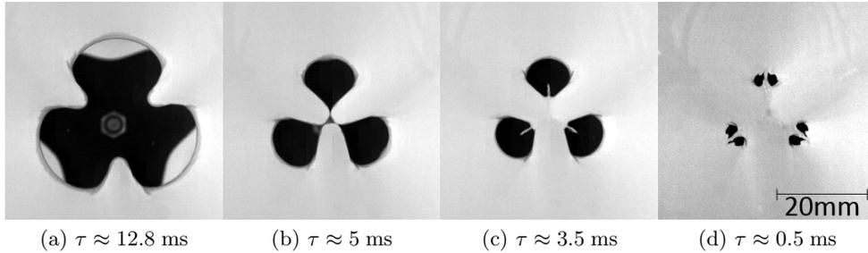
Figure 12: (movie online) Example of sub-cavity formation for an  $m = 3$ ,  $a_3 = 25\%$  collapse. Three large sub-cavities are formed around a smaller central one which quickly disappears. The inward pointing jets in (a) are due to the growth of the initial  $m = 3$  disturbance. The jets in (c) are due to the collision (shown in image b) and subsequent convergence of neighbouring regions of fluid which lead to six small cavities before closing (d).
