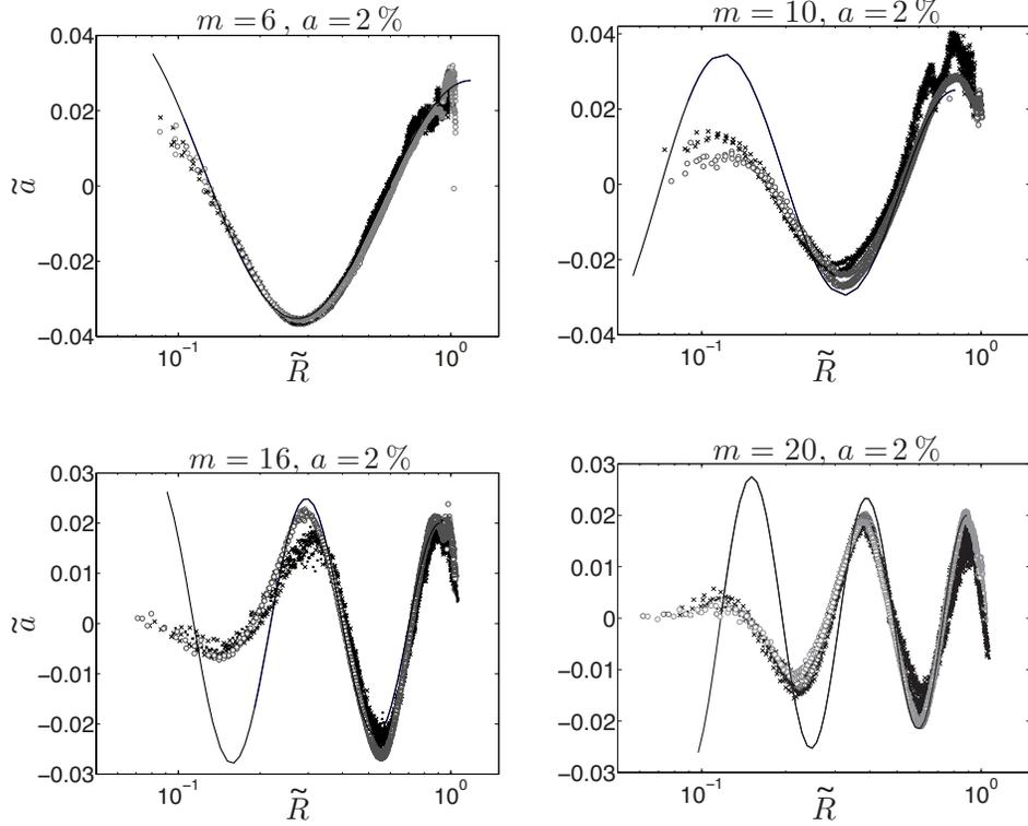
Figure 7: Evolution of the dimensionless oscillation amplitude as the radius collapses. Results for several different mode numbers with a slightly higher initial amplitude of 2% of the mean radius. Circles: measurements with milk, crosses: plain water, solid line: theoretical prediction.
