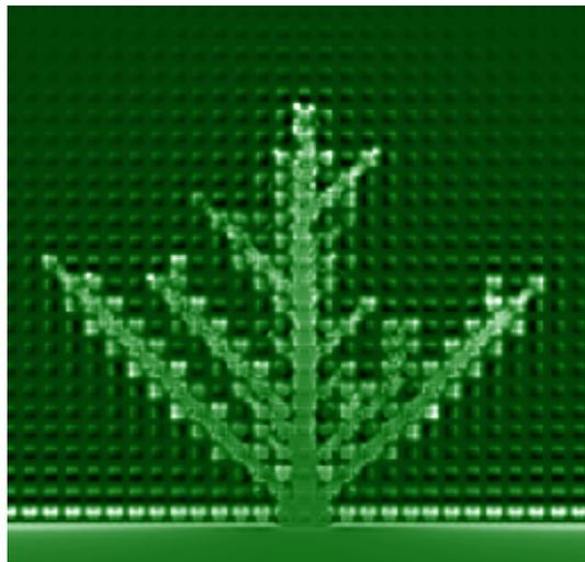
FIG. 3: Results of numerical calculations of the flux penetration into a superconducting film with a square array of square antidots where a thermomagnetic feedback is taken into account. Details of the numerical procedure will be published elsewhere.
