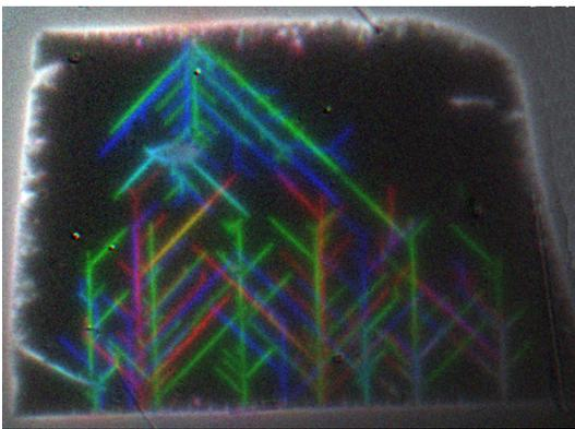
FIG. 2: Overlay of 3 repeated identical MOI experiments showing the flux penetration into the  $a$ -MoGe film, carried out at  $T = 3$  K with  $H = 1.4$  Oe. Each experiment is color coded in red, green and blue, thus the presence of these colors in the overlay shows that the penetration is non-reproducible.
