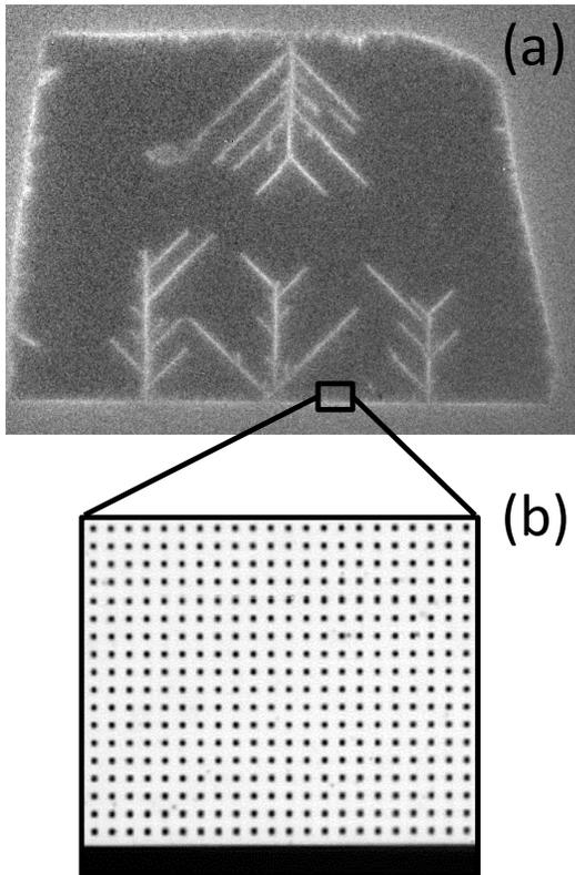
FIG. 1: (a) Magneto optical image of flux penetration at  $T = 4.5$  K and  $H = 1$  Oe, applied perpendicular to the film. The image brightness represents the magnitude of the local flux density. (b) Optical image of the square lattice of square antidots.
