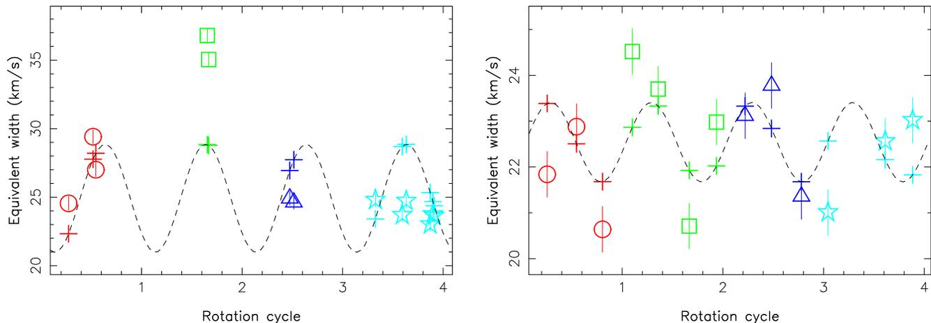
**Figure 8.** Measured (open symbols) and fitted (pluses) equivalent widths of the Ca II IRT LSD profiles of TW Hya in 2008 March (left panel) and 2010 March (right panel). The model wave (dashed line) providing the best (sine+cosine) fit to the data presumably traces rotational modulation, while the deviation from the fit illustrates the strength of intrinsic variability. The open symbols are defined as described in Fig. 3.
