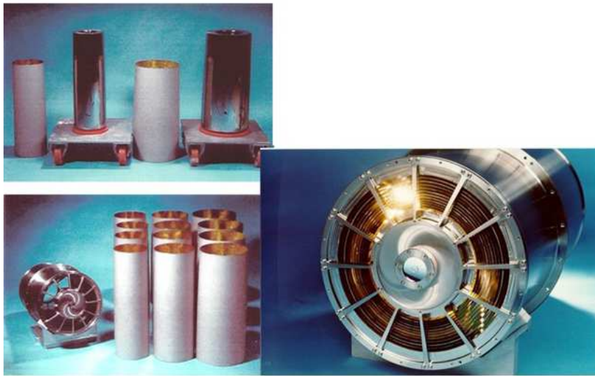
Fig. 13 One of the four mirror modules built for the JET-X telescope (on the right). It consists of 12 nested Wolter-I grazing incidence mirrors held in place by front and rear spiders (see bottom panel on the left side). In the left top panel there are shown also two mandrels used for the electroformation of the shells, together with two shells.
