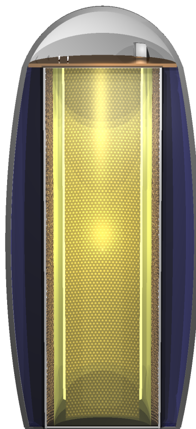
FIG. 1: Artist's view of the LENA detector: The detector tank is 100 m in height and 30 m in diameter. See Fig. 2 for details.
