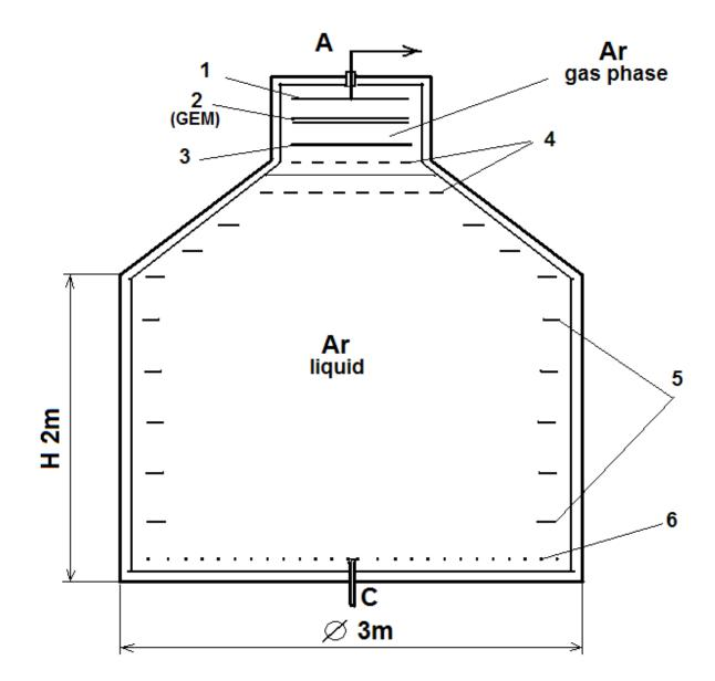
Fig.2. Double-phase Ar chamber: 1-anode, 2-GEM detectors, 3-light screen, 4- grids for electrons transport from liquid Ar to gas phase, 5-the ring electrodes for electric field level, 6-canhode.
