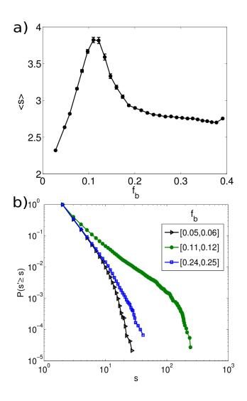
FIG. 5. (Color Online) (a) The average non-giant cluster size as a function of the fraction of broken edges  $f_b$  for the experimental data. (b) The cumulative size distribution for the non-giant components taken at three different ranges of  $f_b$ :  $0.05 \le f_b \le 0.06$  [lower triangles],  $0.11 \le f_b \le 0.12$  [upper circles],  $0.24 \le f_b \le 0.25$  [middle squares].
