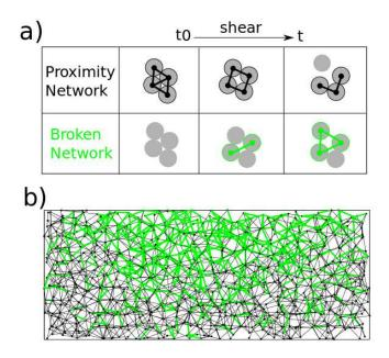
FIG. 3. (Color Online) (a) A schematic of the definition and growth of the broken-links network.b) Example cross section of the broken [green/light gray] and persistent [black] networks, plotted in real space.
