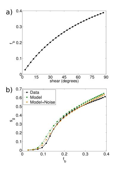
FIG. 4. (Color Online) (a) The fraction of edges broken as a function of applied shear for the experimental data, averaged over all reference networks. (b) The size of the giant component  $s_g$  as a function of the fraction of broken edges for the experimental data [circles], longitudinal strain model [squares], and the longitudinal strain model with noise ( $\eta = 0.82$ ) [triangles]. Errorbars represent the standard error and are smaller than the markers.
