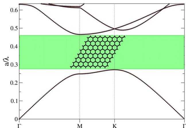
FIG. 1: (Color online) Band structure for the optimal unperturbed TE PBG structure consisting of dielectric walls with dielectric constant  $\epsilon = 11.56$  thickness  $w/a = 0.94$  (shown as an inset), which presents a TE PBG of  $\Delta\omega/\omega_C = 52.63\%$ , the largest known PBG in two-dimensional photonic crystals for this dielectric constant contrast ratio.
