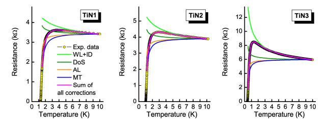
Supplementary Figure S1 Quantum corrections to the conductivity. Theoretical curves describing temperature behavior of quantum corrections to sheet resistance R(T) and their fit to experimental data. Theoretical curves are shown by solid lines and yellow circles represent the experimental data.
