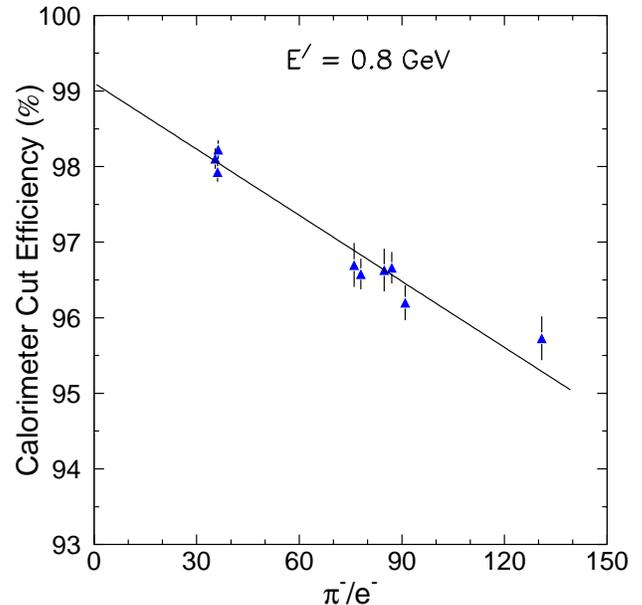
FIG. 7: (Color online) The electromagnetic calorimeter cut efficiency versus  $\pi/e$  ratio. The fit represented by the solid line extrapolates the efficiency at zero  $\pi/e$  ratio in order to obtain the true electron efficiency.
