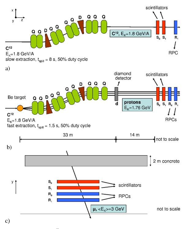
**Figure 4.** a) Setup for focused C<sup>12</sup> irradiation (kinetic energy  $E_K = 1.8 \text{ GeV/A}$ ,  $\sigma_{E_K}/E_K < 1\%$ ). b) Setup for diffuse proton irradiation ( $E_K = 1.76 \text{ GeV}$ ,  $\sigma_{E_K}/E_K = 4\%$ ) after C<sup>12</sup> reactions in a secondary Beryllium target placed 33 m upstream the experimental hall. Diamonds have been added and also a second RPC ( $R_o$ ). c) Setup for cosmic muon detection.
