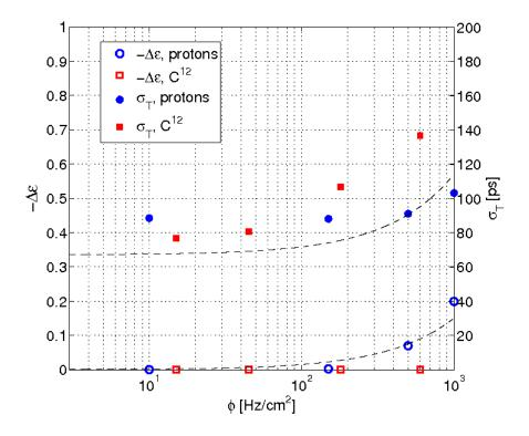
**Figure 13.** Time resolution  $\sigma_T$  and decrease in efficiency  $-\Delta\varepsilon$  in the RPCs for protons at  $E_K = 1.76 \pm 4\%$  GeV (circles) and fully stripped Carbon ions at  $E_K = 1.8$  GeV/A (squares) as a function of their flux. The operating voltage was V = 5.6 kV.
