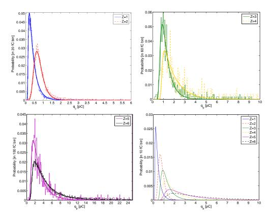
**Figure 11.** Up-left: RPC charge distributions for fully stripped ions with atomic charges Z = 1,2 together with a fit to a Landau-like function. Up-right: Z = 3,4. Down-left: Z = 5,6. Down-right: Fitted curves for Z = 1-6. The normalized momenta is  $\gamma\beta \simeq 2.7$  in all cases, V=5.6 kV and  $\phi < 10$  Hz/cm<sup>2</sup>.
