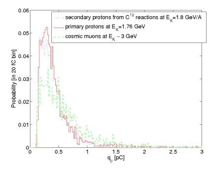
**Figure 9.** Comparison of the charge distribution measured in the RPC under a diffuse proton beam at a kinetic energy  $E_K = 1.76 \text{ GeV} \pm 4\%$  (continuous line), secondary forward protons from C<sup>12</sup> interactions at  $E_K \sim 1.8 \text{ GeV}$  (dotted) and cosmic muons at  $E_K \sim 3 \text{ GeV}$  (dashed).
