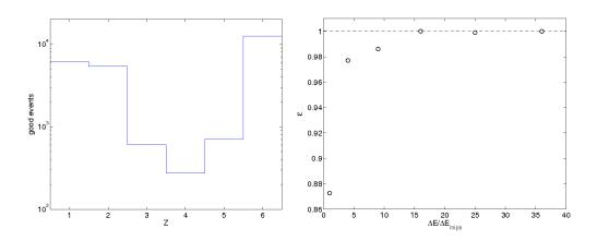
**Figure 16.** Left: population of ions with charge states 1 - 6 after cuts ('good events'). Right: detection efficiency as a function of the energy loss expressed in mips units. The points have being obtained for V = 5.6 kV at low particle rates ( $\phi < 10$  Hz/cm<sup>2</sup>).
