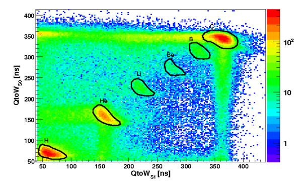
**Figure 7.** Two-dimensional correlation plot between the raw signal widths obtained in the reference scintillators after offset subtraction (color on-line). Six blobs can be identified being the most prominent ones attributable to protons, He and  $C^{12}$ . The other 3 blobs with a much lower yield must be Li, Be and B or charge states of the  $C^{12}$  ion.
