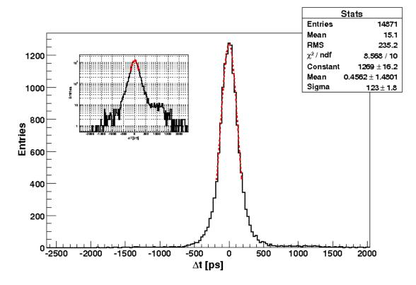
**Figure 10.** Time of flight distribution between RPCs for a diffuse proton beam (kinetic energy  $E_K = 1.76 \text{ GeV} \pm 4\%$ ) at 150 Hz/cm<sup>2</sup> and V=5.6 kV. The inset shows the same distribution in logarithmic scale, indicating the presence of tails at 1% level. The counter resolution from the fit is  $\sigma_T = 123/\sqrt{2} = 87\text{ps}$ .
