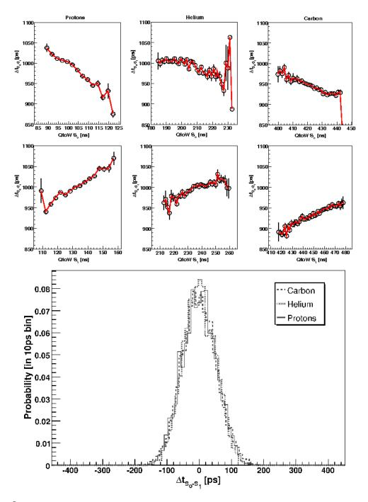
**Figure 8.** Up: multi-linear fit used for correcting the walk of the time of flight between the reference scintillators  $(\Delta t_{S_o-S_1})$  as a function of the signal width (*QtoW*) for p, He and C<sup>12</sup>. Down: distribution of times of flight between scintillators after the correction procedure for the three species.
