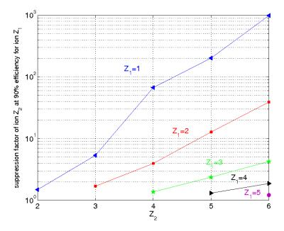
**Figure 17.** Suppression factor of element in charge state  $Z_2$  when imposing a cut in the RPC charge for a 90% identification efficiency of element in charge state  $Z_1$ . The suppression factor has been obtained after fitting the charge distributions to Landau-like functions.
