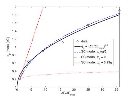
**Figure 19.** Measured charge at maximum  $q_p(\max)$  as a function of the energy lost in mips units (circles). The  $\sqrt{\Delta E}$  experimental scaling is shown together with the evaluation of the model of Fonte [15] under the assumptions of the text, for three different positions  $x_o$  of the avalanche inside the gap (center, close to the cathode and close to the anode).
