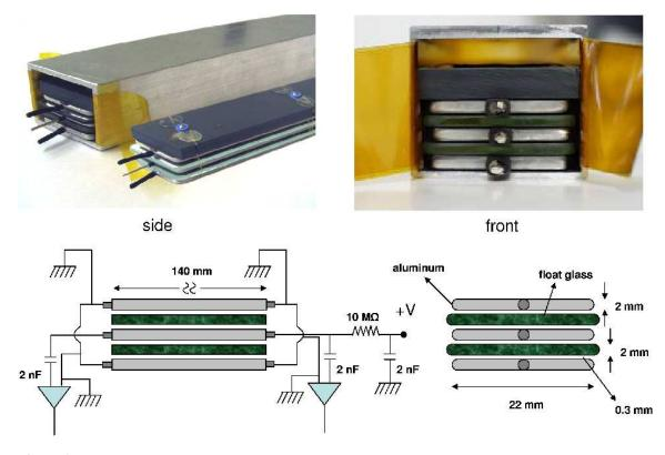
**Figure 1.** Up: pictures showing a typical HADES cell, before and after being placed in its corresponding Faraday cage. Down: side and front sketch of a HADES cell together with the electrical scheme used for these measurements.
