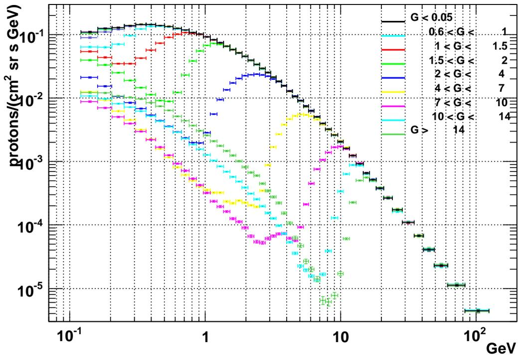
Fig. 5. Plot of the differential energy spectrum of PAMELA at different values of geomagnetic cutoff  $G$ . It is possible to see the primary spectrum at high rigidities and the reentrant albedo (secondary) flux at low rigidities. Only statistical errors are shown.
