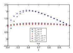
Fig. 2. Approximate  $T_0(r) + \epsilon T_1(r)$  temperature profiles for different  $\mu$  (= -4, -1, 1) with  $\delta = 2$ . Here, the wave number of roughness k is equal to 8,  $\epsilon = 0.1$ ,  $\beta = \pi/4$  and the inner boundary is s = 0.4. We can observe that the small-amplitude wavy-roughness changes the near-inner-wall temperature distribution significantly once  $\mu = -4$ .
