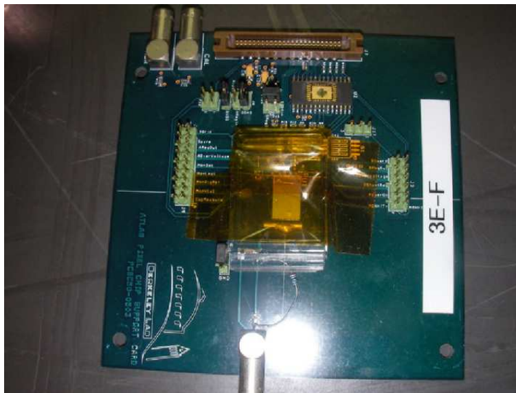
Fig. 75: Picture of the 3D-ATLAS pixel assemblies mounted on one of a pcb testboard with a protective cover.
