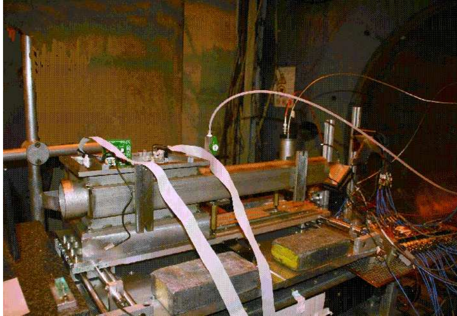
Fig. 79: FP420 2007 test beam setup including one movable station, two blades, and two timing detectors (one GASTOF and two QUARTICS).
