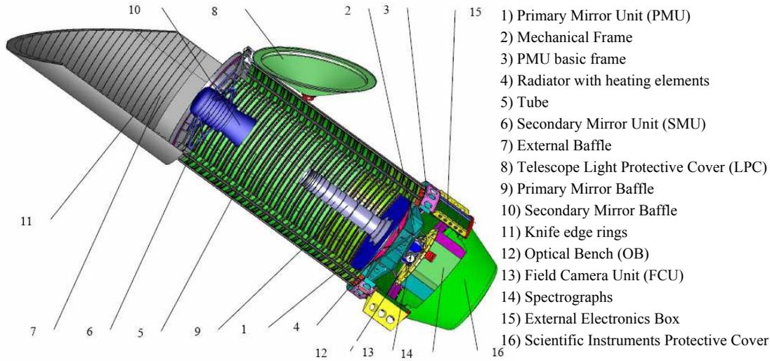
**Fig. 1** General view of the T-170M telescope.
