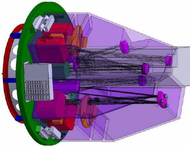
**Fig. 3** Schematic overview of HIRDES (Kappelmann et al. 2006).
