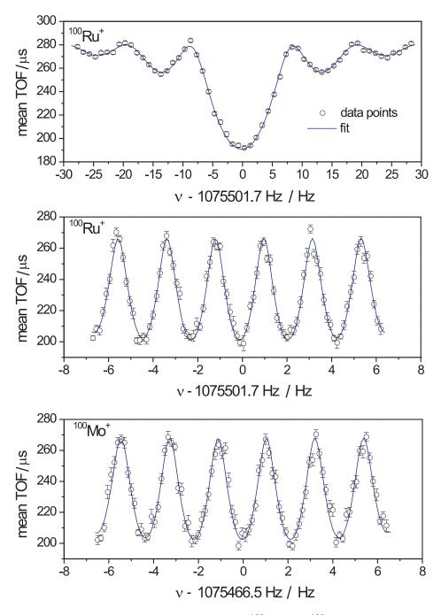
Fig. 2. Time-of-flight (TOF) resonances of  $^{100}$ Ru and  $^{100}$ Mo ions from the precision trap. The top panel represents a typical TOF resonance using the conventional excitation scheme with an excitation time of 100 ms. The middle and bottom panels display the TOF resonances for  $^{100}$ Ru and  $^{100}$ Mo ions using the Ramsey excitation pattern with 50-400-50 ms, respectively.
