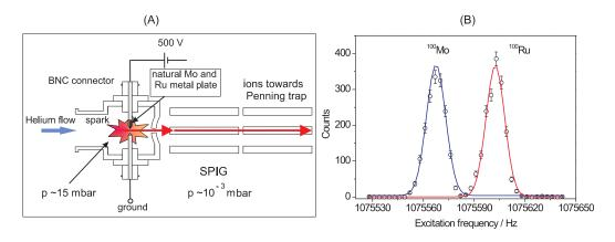
Fig. 1. (A): Schematic drawing of an off-line ion source to produce a variety of stable and long-lived mixed singly-charged ion beams. (B): Mass spectrum of ions ejected from the purification trap after buffer gas cooling for mass region A = 100. A gaussian fit to the data yields a FWHM of about 11 Hz, which corresponds to a mass resolving power of about  $1 \times 10^5$ .
