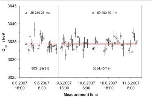
Fig. 4. Q-values obtained from individual measurements of <sup>100</sup>Mo in June 2006 by using <sup>100</sup>Ru as a reference. Triangles and circles correspond to different excitation times (see legend). The data collection was stopped every night before the automatic  $B_0$  dump at 3:00 AM. The statistical, count-rate and magnetic-field fluctuation uncertainties have been taken into account for each set.
