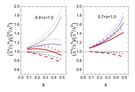
FIG. 9: (Color online) The production ratio of  $(\bar{\Lambda}^A/\Lambda^A)/(\bar{\Lambda}^D/\Lambda^D)$  at  $Q^2 = 5$  GeV<sup>2</sup>, calculated in 0.7 < z < 1.0 and 0.4 < z < 1.0. The solid, dashed and dotted curves are the predictions of the cluster model, the rescaling model and the pion excess model respectively. The thin, normal and thick curves correspond to the three options of the fragmentation (1), (2), (3) respectively. The target nuclei assumed here is Fe.
