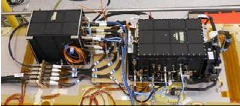
Figure 4.8: Poseidon-3C processing unit (PCU) and radio frequency unit (RFU). Copyright CNES - Thales Alenia Space.
