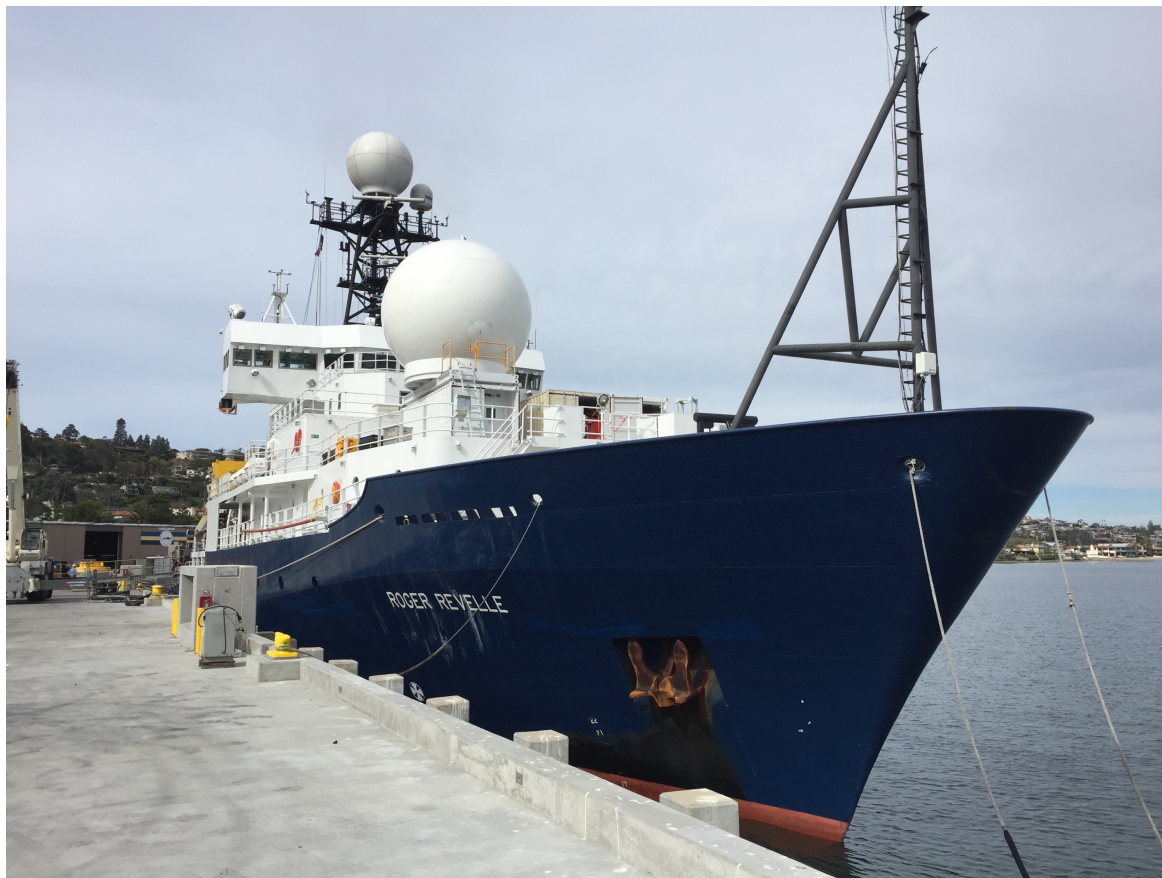
Fig. 1. Picture showing the SEA-POL radar installed on the forward 02 deck of the R/V Roger Revelle.
