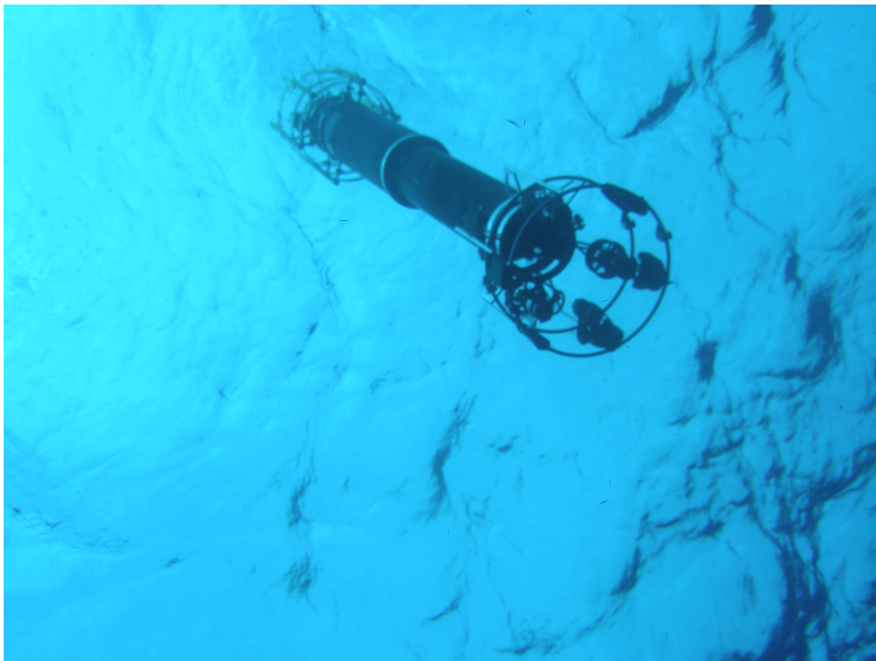
Figure 1: Photograph of the Air-Sea Interaction Profiler (developed in the AirSea Group at NUI, Galway) ascending towards the ocean surface where it records the small-scale processes with high-resolution sensors.
