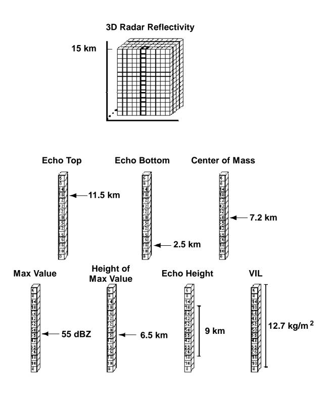
Figure 7. Reflectivity products derived from pencil-beam radar reflectivity.
