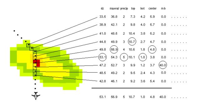
Figure 11. Data are extracted from Cartesian bins occupied by the aircraft. One value of each variable is selected to characterize the penetrations.
