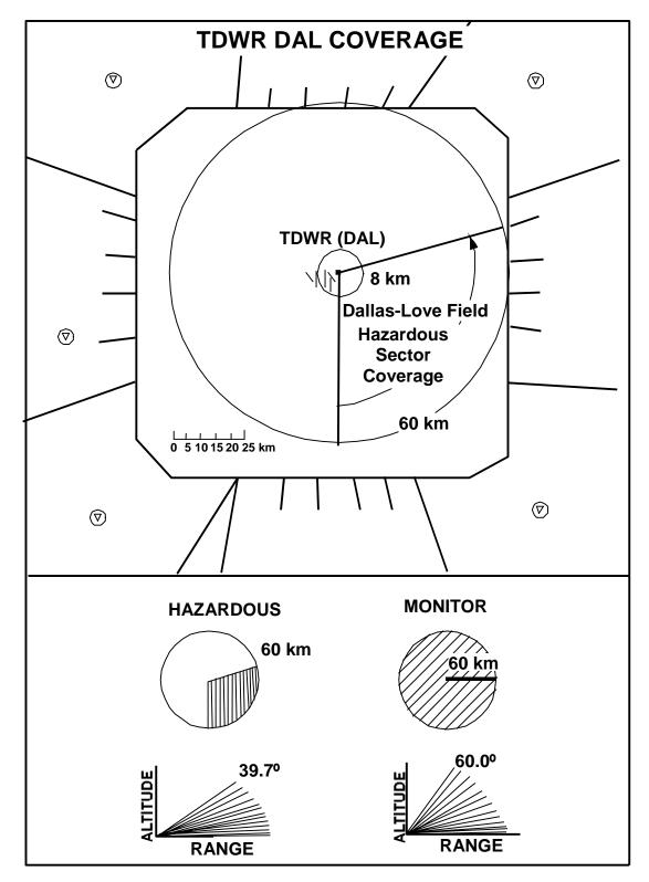
Figure 9. The location and coverage region for the DFW TDWR. Data were used beyond 10km and within 60 km of the radar. The lower Figure shows a plan view of the scanning range and a vertical cross section of the scan strategy for the radar in "hazardous" and "monitor" modes.
