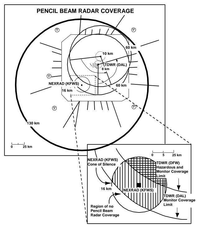
Figure 14. Pencil-beam radar coverage regions inside the TRACON.
