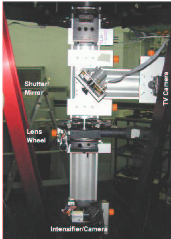
Figure 3.8: The Imperial College SCIDAR instrument mounted at the Calar Alto 1.23 m telescope.
