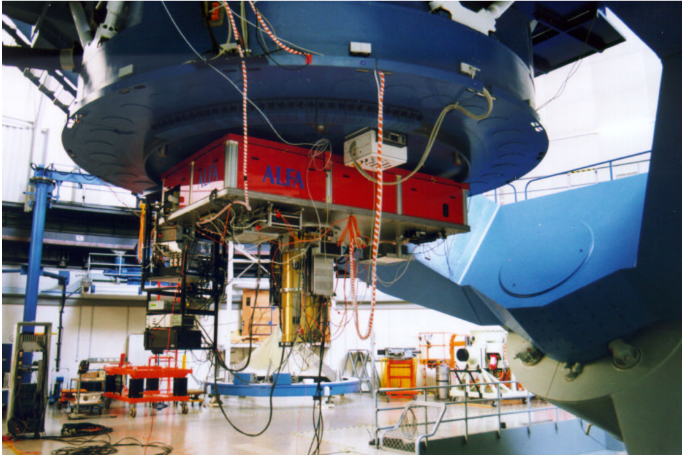
Figure 3.7: ALFA and Omega Cass mounted at the Cassegrain Focus of the Calar Alto 3.5 m telescope.
