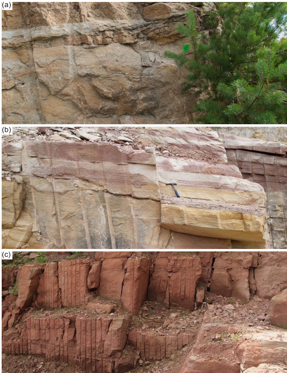
Figure 5: (a) Pervasively bleached sandstone, white to yellowish-brown colour. Typical “Haardtrand Fazies”. The colours follow the bedding planes. Vertical scale is approximately 1 m. Lower Buntsandstein (Rehberg-Sch.), quarry Hanbuch, Neustadt a.d.W. (b) Yellow, red and white sandstones. The colours follow the bedding planes. White bleaching zones are best developed around fractures. Lower Buntsandstein, Cleebourg. (c) Red sandstone with minor bleached layers, hardly visible on the weathered surface. This is the most common appearance of the Buntsandstein in South Germany. Vertical scale is approximately 3 m. Lower Buntsandstein, Rockenau.
