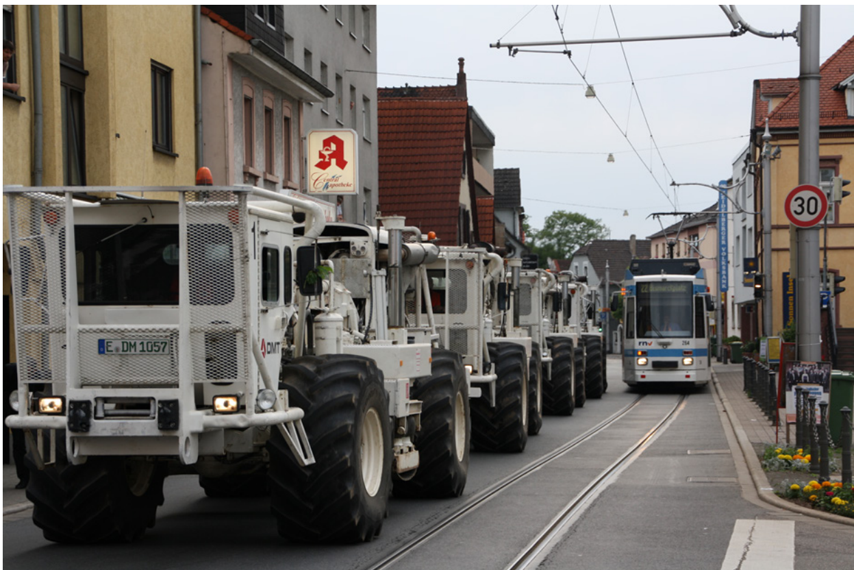
Fig. 5: Four-source vibroseis pattern acquiring data in a densely populated area. 2D-seismic-survey Heidelberg 2010 (WENKE et al., 2012a).
