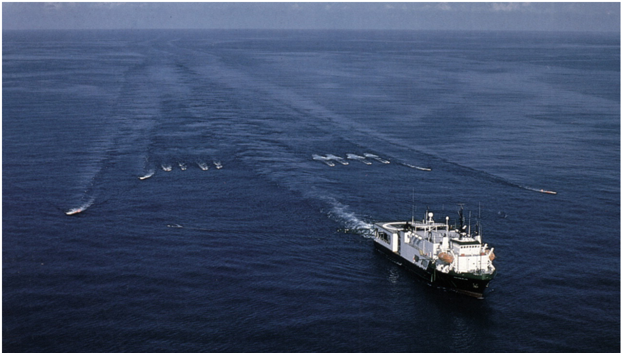
Fig. 6: Marine seismic acquisition unit including vessel with airgun and recording and the pulled streamer (receiver) arrays (DRAGOSET, 2005).
