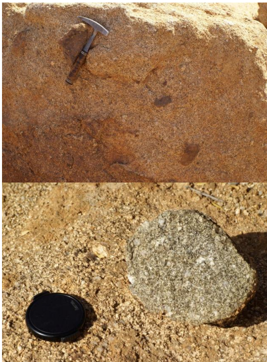
Fig. 2.31: Precambrian granite (600 Ma) at Tarsouale (MA-12). (A) Mafic xenoliths (Gabbro) in granite. (B) Hand specimen of the porphyric granite.
