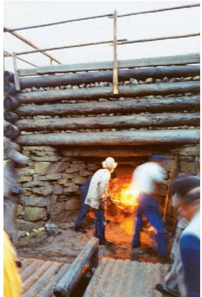
Fig. 4. Making iron in the reconstructed blast furnace at Lapphyttan, Norberg. Photo: Hans Lind (f)
