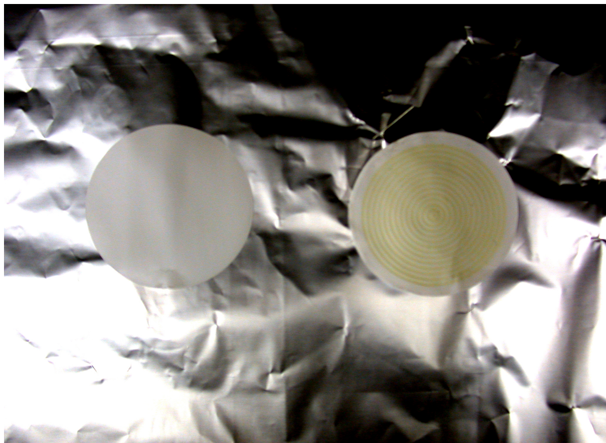
Photo. S1. Sample filter obtained in the experiment (run 3) with benzene (right) and blank filter (left); in contrast, a sample filter obtained in the experiment with 1,3,5-TMB was white.
