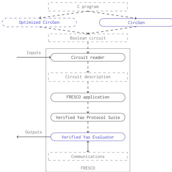
**Figure 1: Verified cryptographic software stack. Blue rectangles identify the verified components of the stack, while black rectangles represent part of our trusting computing base. Dashed blue rectangles are partially verified elements and in dashed black rectangles one can find intermediate input/output items.**
