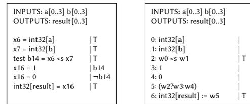
**Figure 9: Guarded instructions instead of control-flow (left) and corresponding SSA conversion (right).**
