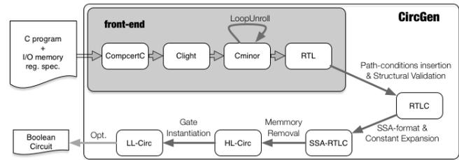
Figure 6: Architecture of the certified compiler CircGen
