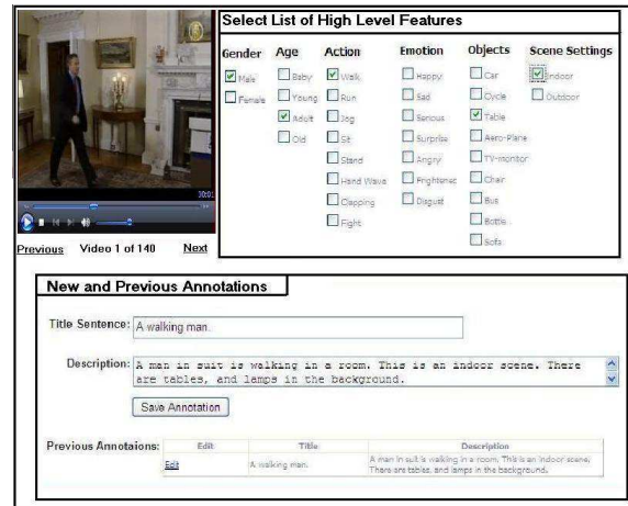
Figure 1: Video Description Tool (VDT) . An annotator watches one video at one time, selects all HLFs present in the video, describes a theme of the video as a title and creates a full description for important contents in the video.
