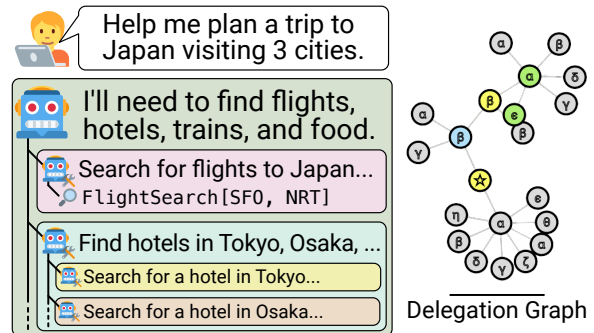
Figure 1: ReDel allows developers to create systems of recursive agents, inspect each agent’s state, and visualize a system’s delegation graph (right). Recursive agents can be used to solve complex tasks, such as planning a trip to Japan (left).
