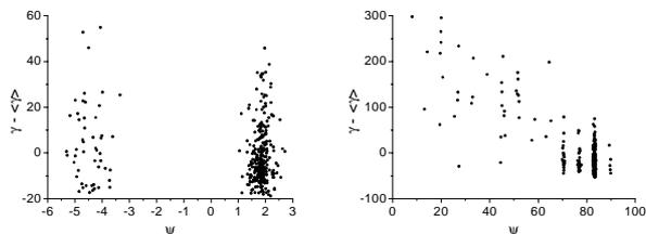
Figure 6: Phase portraits of bunches at  $z \approx 200$  m for  $\delta\varphi = 0$  (left) and  $\delta\varphi = 0.5\pi$  (right).
