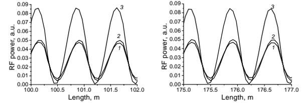
Figure 3: Spatial dependences of microwave power in two driver fragments for negative phase advance per cell: 1 –  $\delta\varphi = 0$ ; 2 –  $\delta\varphi = -0.1\pi$ ; 3 –  $\delta\varphi = -0.5\pi$ .
