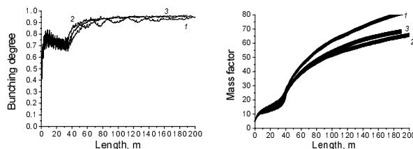
Figure 8: Spatial distributions of the bunching degree (left) and main bunch energy (right) for  $\delta\varphi = 0.5\pi$  depending on the particle number in the simulation: 1 –  $N_p = 100$ , 2 –  $N_p = 200$ , 3 –  $N_p = 400$ .
