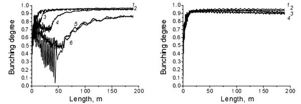
Figure 4: Spatial distributions of bunching degree. Left: 1 –  $\delta\varphi = 0$ ; 2 –  $\delta\varphi = 0.1\pi$ ; 3 –  $\delta\varphi = 0.4\pi$ ; 4 –  $\delta\varphi = 0.5\pi$ ; 5 –  $\delta\varphi = 0.7\pi$ ; 6 –  $\delta\varphi = \pi$ . Right: 1 –  $\delta\varphi = 0$ ; 2 –  $\delta\varphi = -0.1\pi$ ; 3 –  $\delta\varphi = -0.5\pi$ ; 4 –  $\delta\varphi = -\pi$ .
