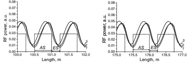
Figure 2: Spatial dependences of microwave power in two driver fragments for positive phase advance per cell: 1 –  $\delta\varphi = 0$ ; 2 –  $\delta\varphi = 0.1\pi$ ; 3 –  $\delta\varphi = 0.5\pi$ . Locations of the accelerating sections and power extraction sections are marked as ‘AS’ and ‘ES’.
