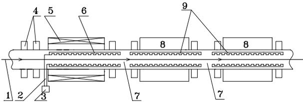
Figure 1: TBA driver scheme: 1) electron beam; 2) waveguide; 3) magnetron; 4) focusing magnetic lenses; 5) solenoid; 6) TWT – beam buncher; 7) sections of RF power extraction; 8) accelerating sections; 9) corrugated waveguide – slowing electrodynamic structure.
