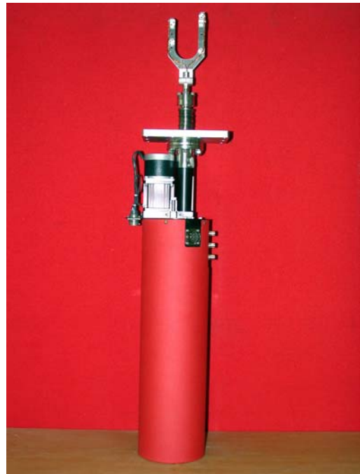
Fig. 1. (color) Photograph of a 6-inch stroke actuator.
