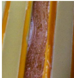
Figure 11. Cable positioning error
