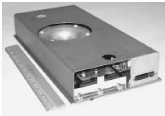
Figure 4. Solid-state switch plate for the Argonne Advanced Photon Source. Each plate is rated at 3.3 kV, 100 A continuous; 36 plates are connected in series to achieve over 100 kV switch capability.
