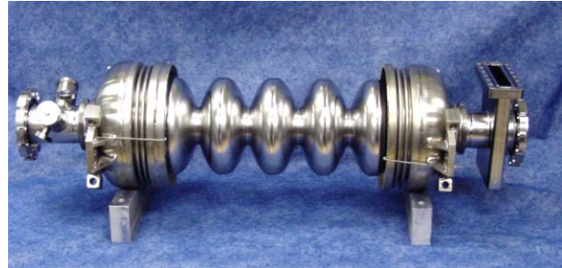
Figure 1: JLab "OC" shape, 1.5GHz, 7-cell niobium cavity with helium vessel removed.
