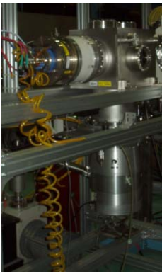
Figure 2. Picture of the installed ion injector. The vacuum system consists of gate valve, TMP with rotary pump and penning gauge.
